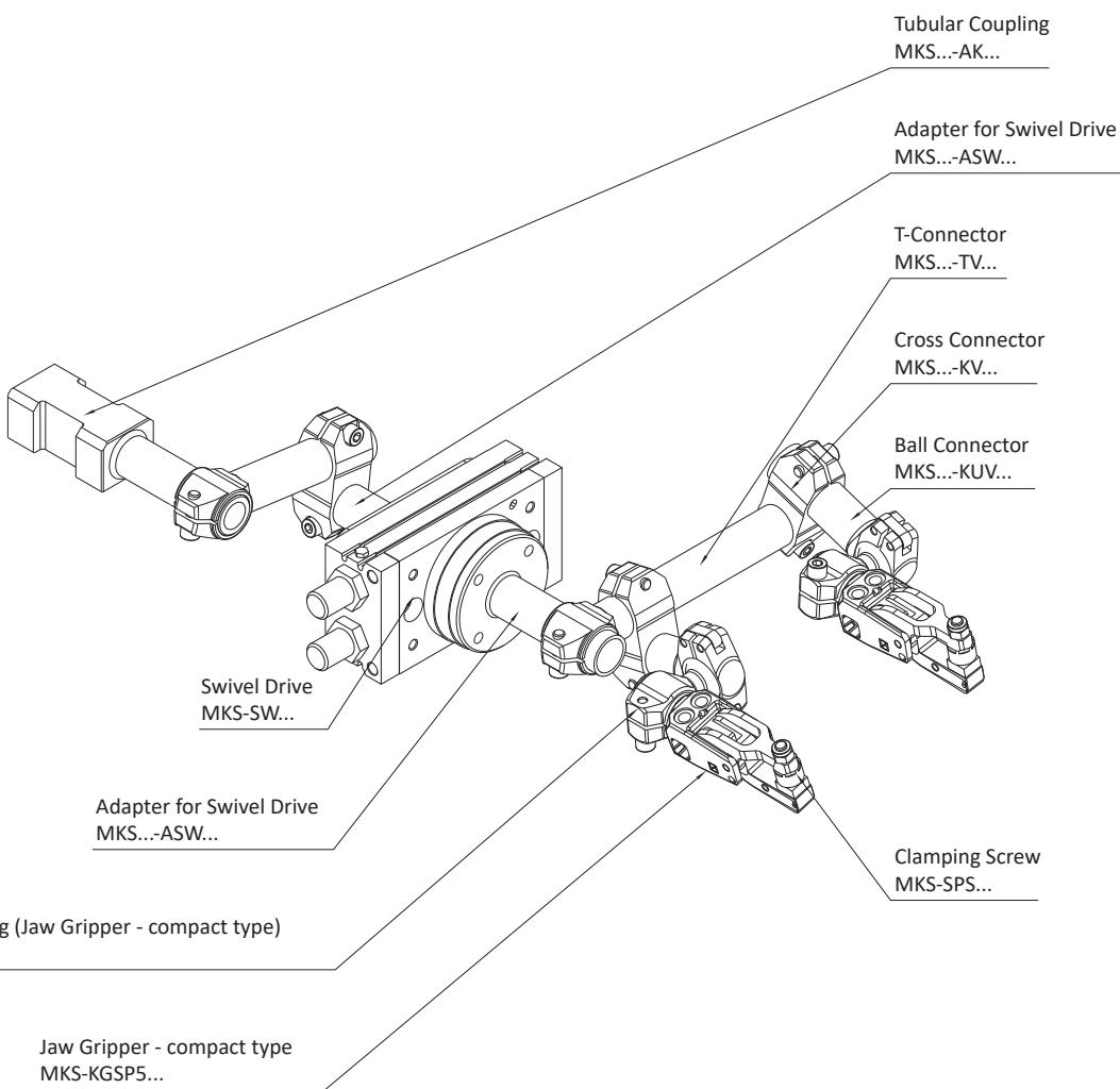
TMZ-Assembly with Dovetail Coupling and Jaw Gripper (compact type)
