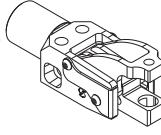
Type: body aluminium, clamping orientation 0°, clamping type wide, with sensor preparation IDS19, clamping lever arm up for clamping screw, clamping lever arm down plain for sensor, ports (P) G1/8
