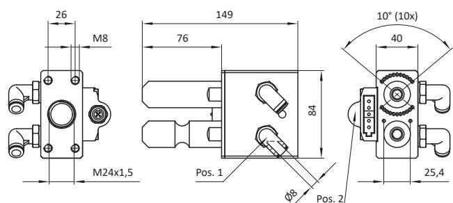
Technical drawing of MKS-GAK04-X2 coupling detail showing side view dimensions: 26 mm width, 149 mm height, 76 mm depth, and M8 thread.
