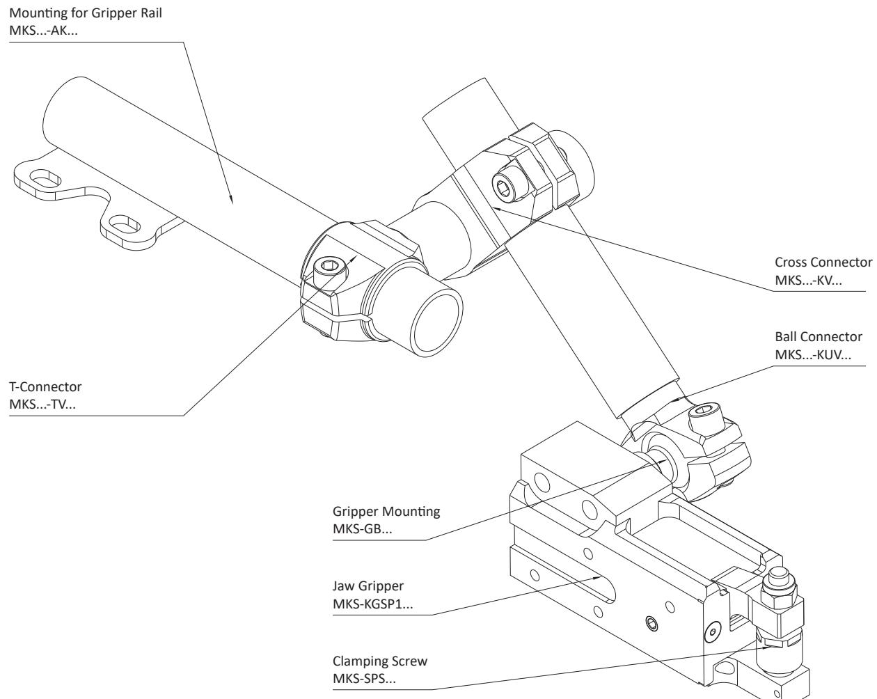
**TMZ-Assembly for Gripper Rail with Jaw Gripper - (compact type)**
