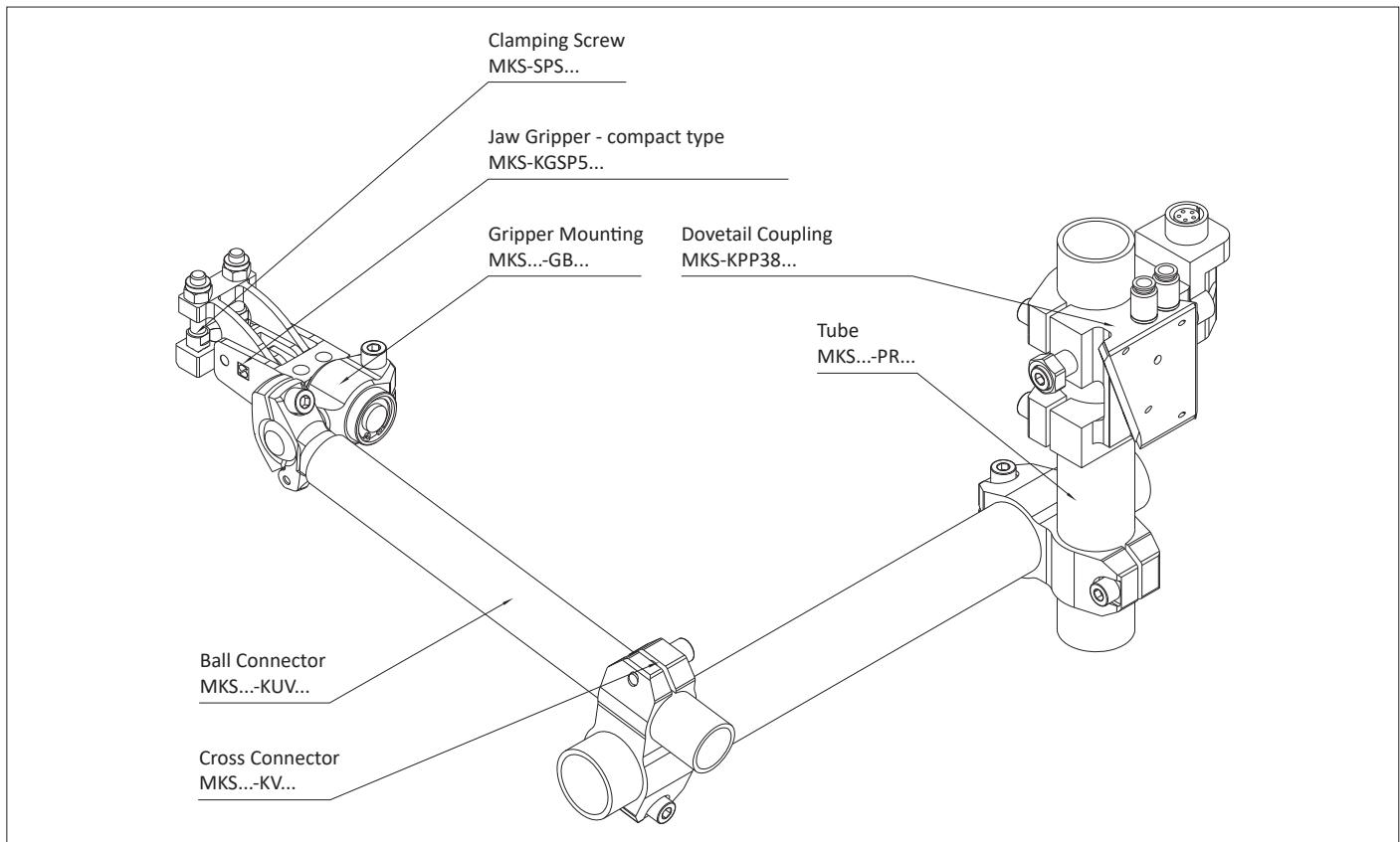
**TMZ-Assembly with 2-Channel-Coupling, Jaw Gripper and Transport Paddle**
