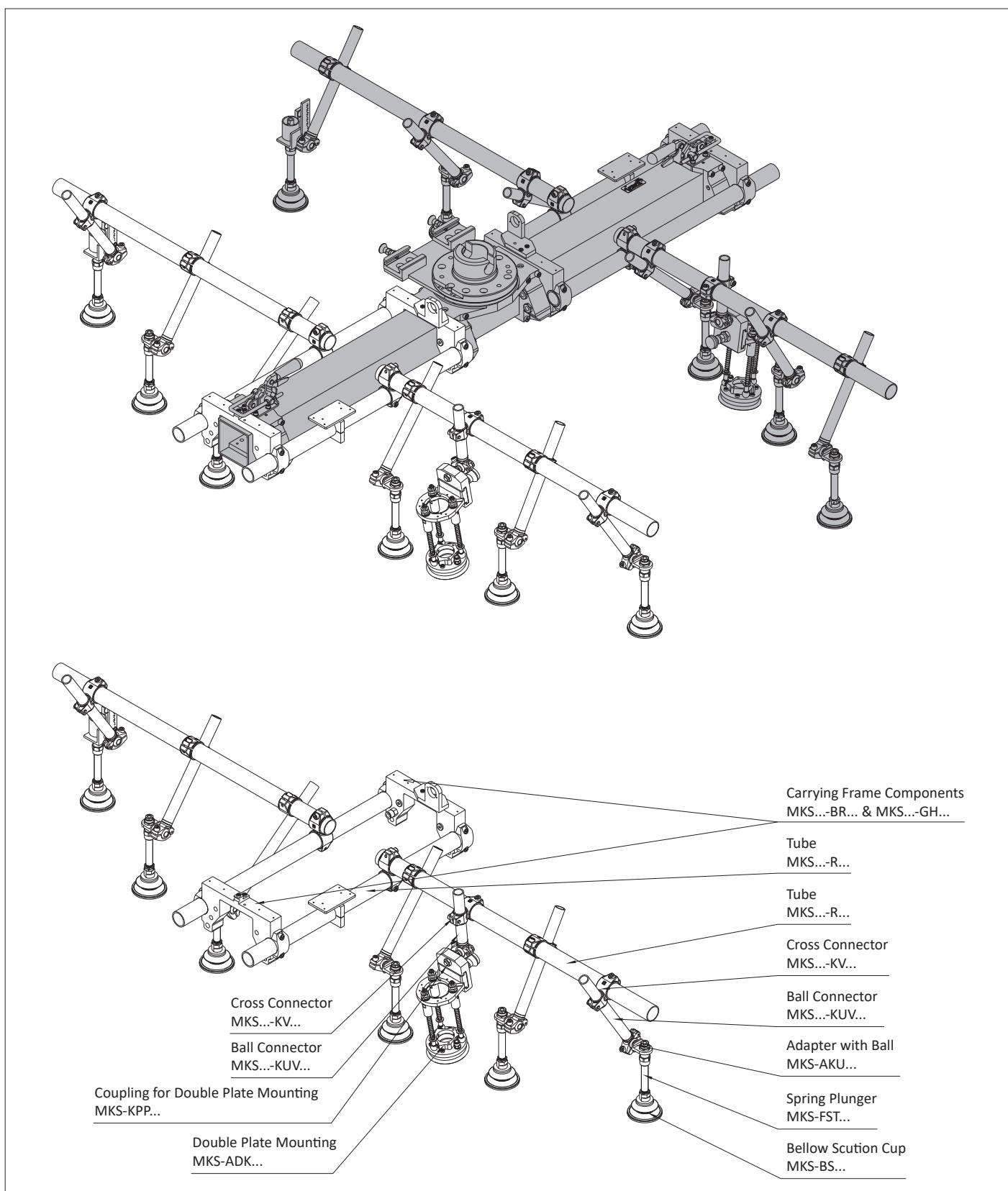
TMZ-Assembly - Destack-Tooling for Hot Forming
