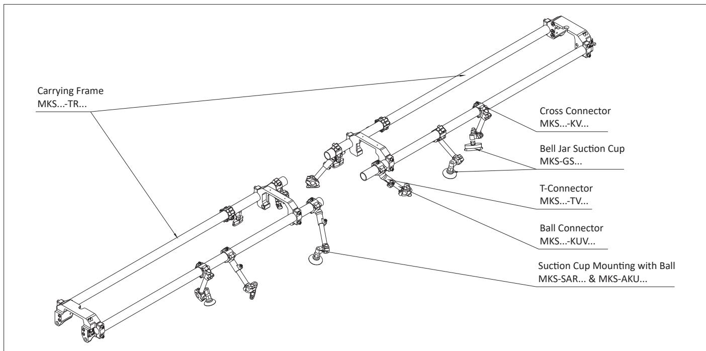
**TMZ-Assembly - Unload Feeder for Hot Forming**
