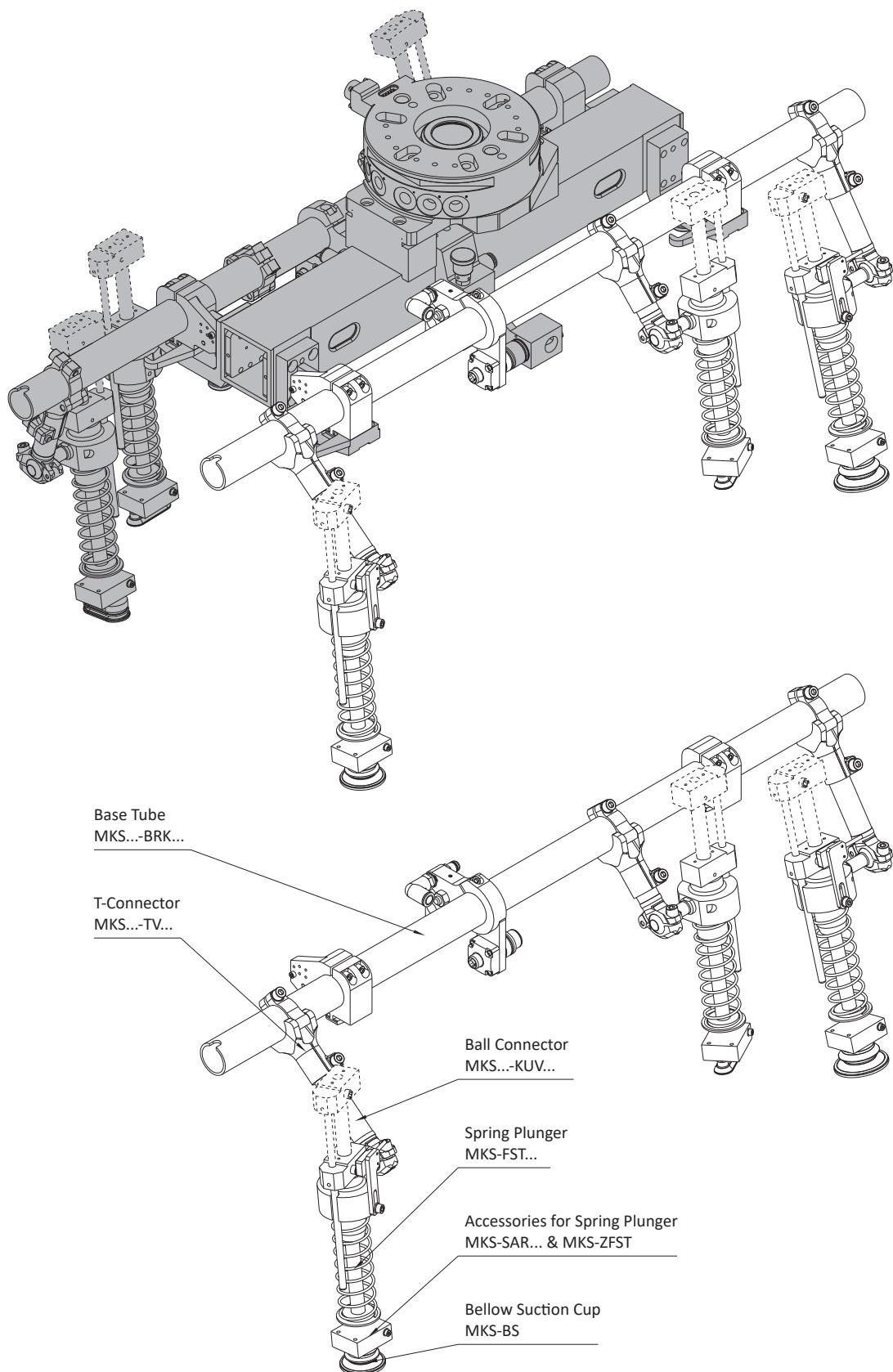
TMZ-Assembly - Tooling for Bayonet-Coupling with Spring Plungers
