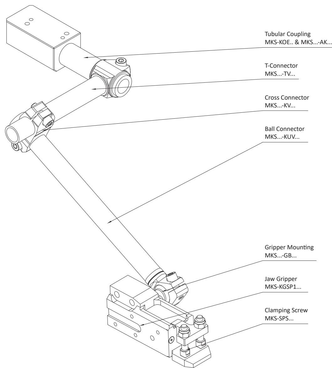
**TMZ-Assembly for Tubular with Jaw Gripper (compact type)**
