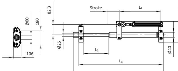
Front view technical drawing of the slide unit showing overall dimensions and stroke length.
