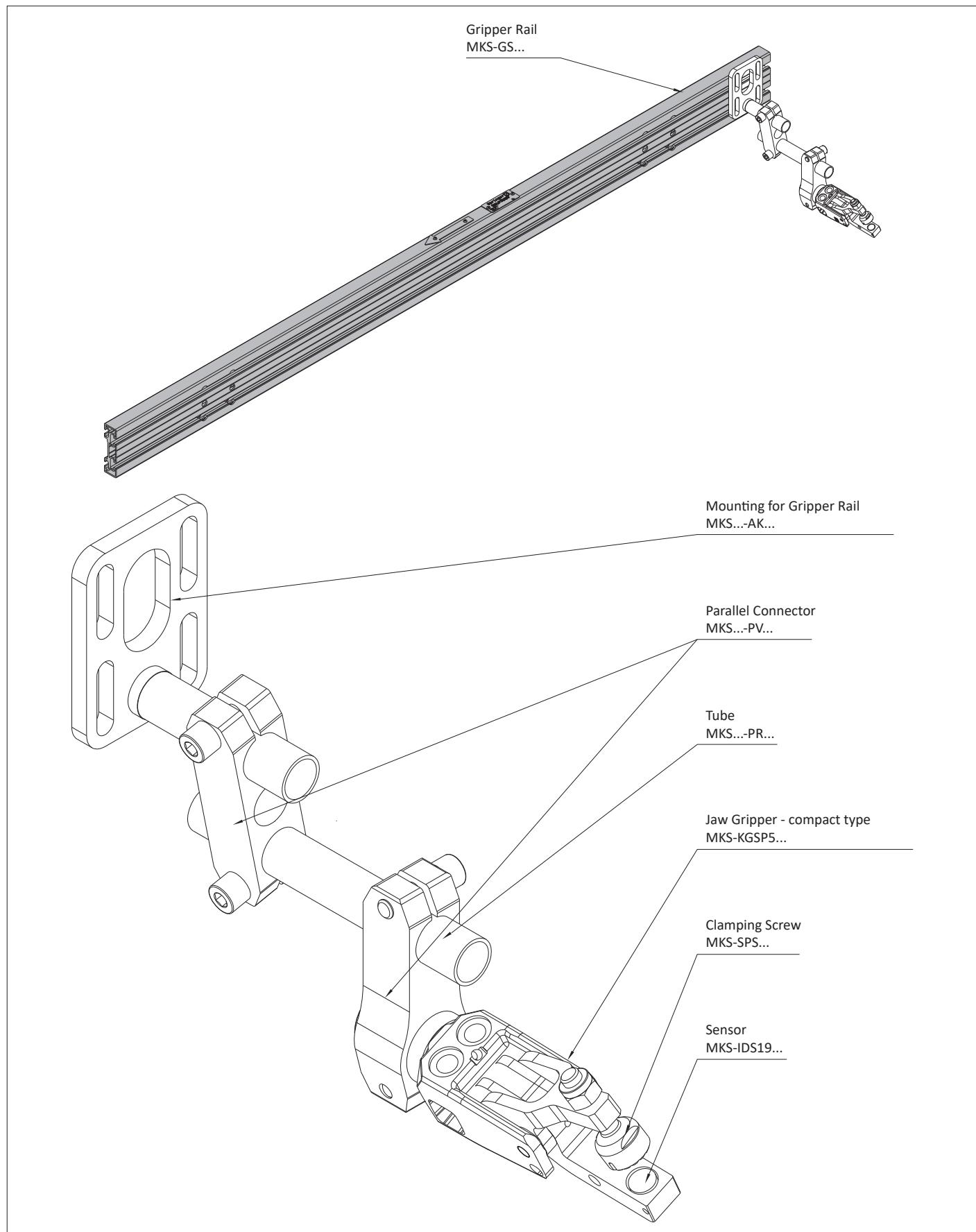
**TMZ-Assembly for Tubular with Jaw Gripper**
