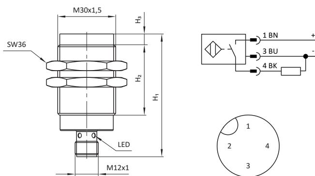
Type: for swivel drive, for groove, PNP / NO, M12-connector
