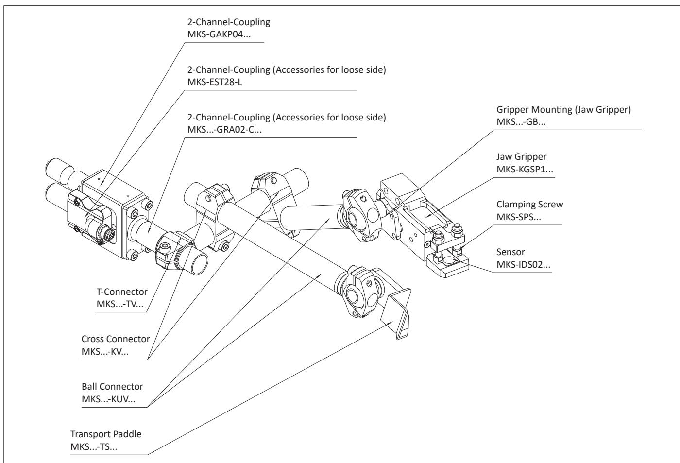
TMZ-Assembly - Double Tube Tooling
