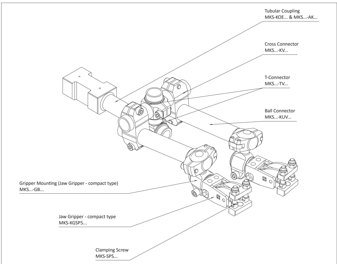
**TMZ-Assembly with Swivel Drive and two Jaw Grippers (compact type)**
