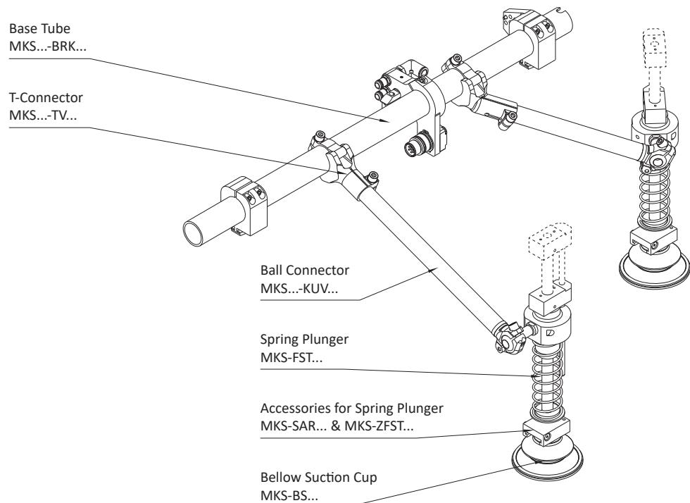
TMZ-Assembly - Robot-Press-Tooling
