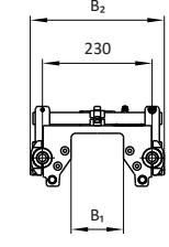
Side view technical drawing of the slide unit showing side dimensions and stroke length.
