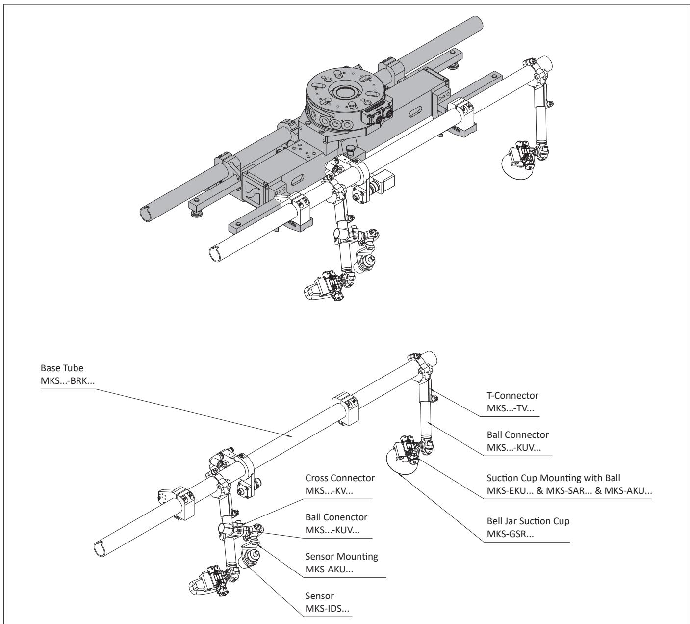
**TMZ-Assembly - Tooling Finished Part Stacking System**
