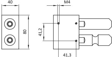
Technical drawing of MKS-GAKP05-2-LB coupling detail showing side view dimensions: 40 mm width, 80 mm height, 41,2 mm depth, 41,3 mm height, and M4 thread.
