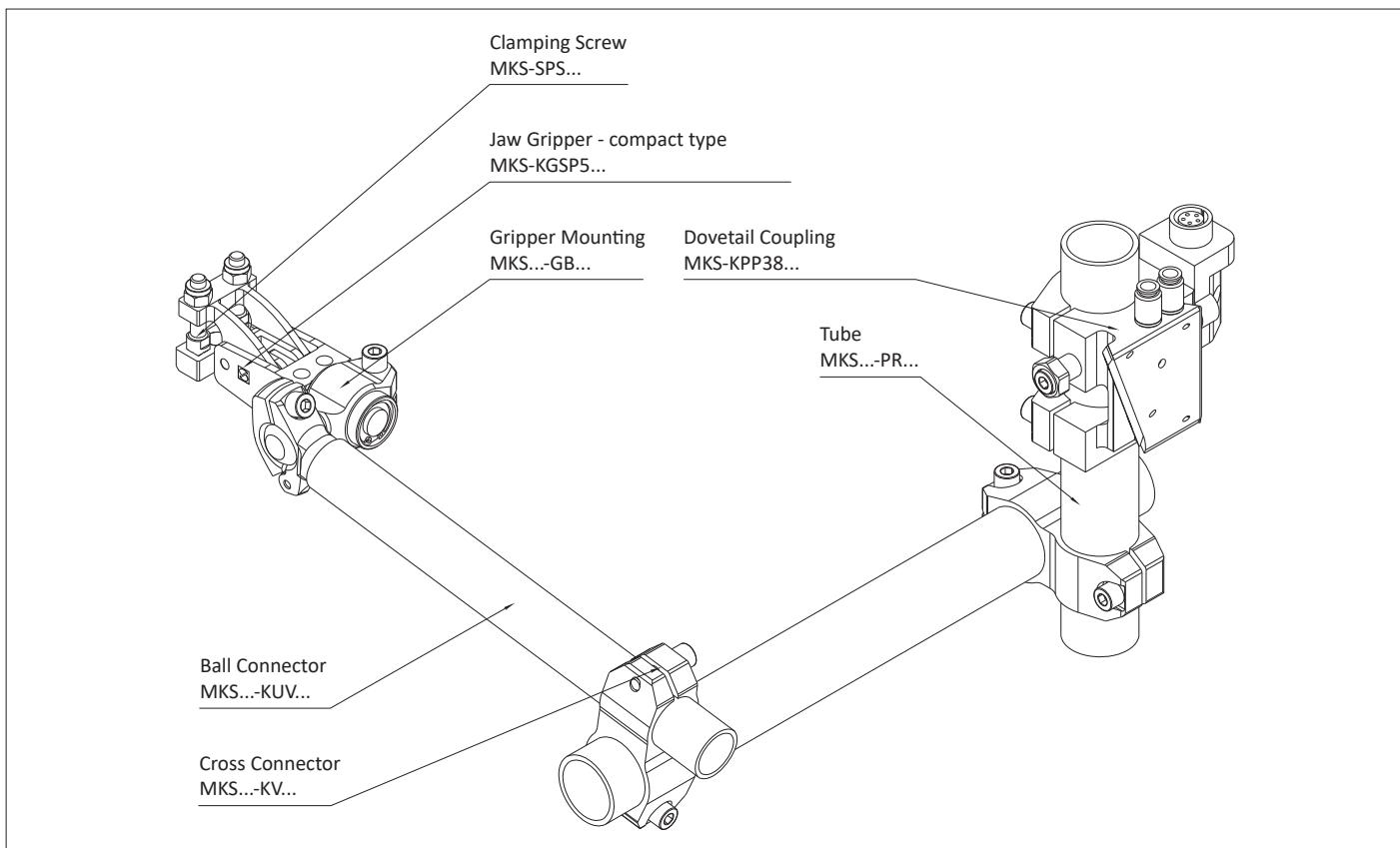
**TMZ-Assembly with 2-Channel-Coupling, Jaw Gripper and Transport Paddle**
