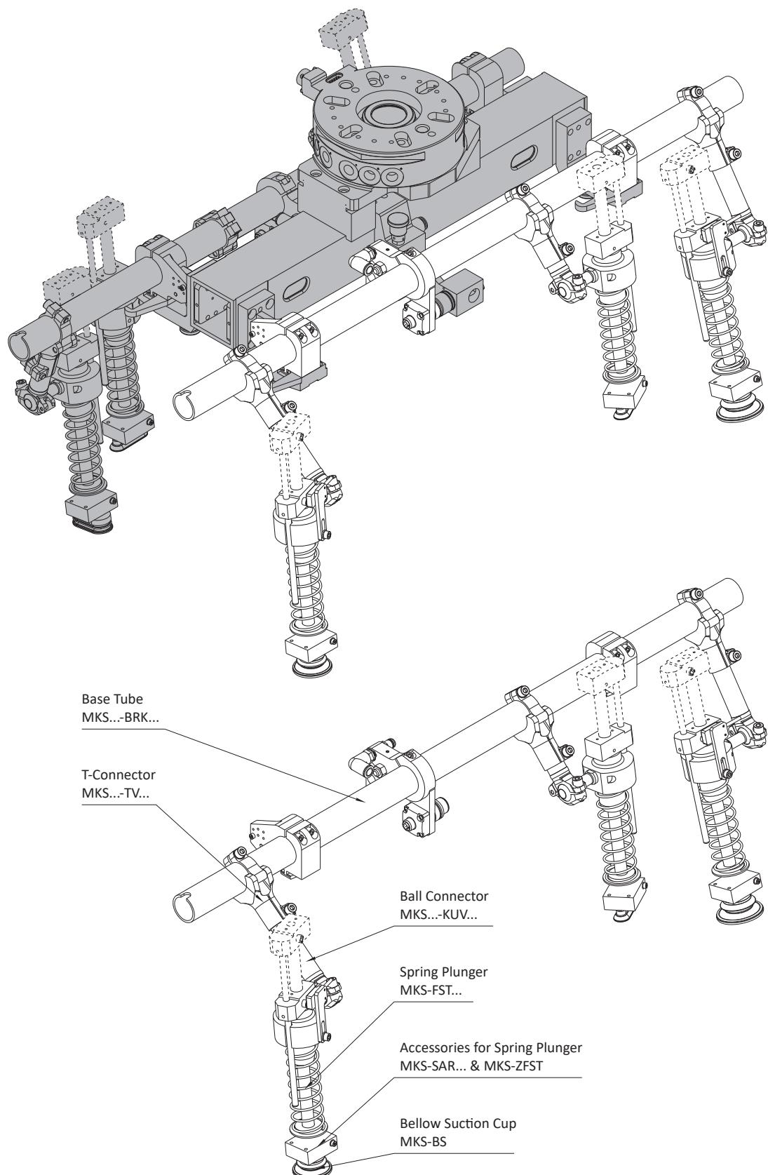
**TMZ-Assembly - Tooling for Bayonet-Coupling with Spring Plungers**
