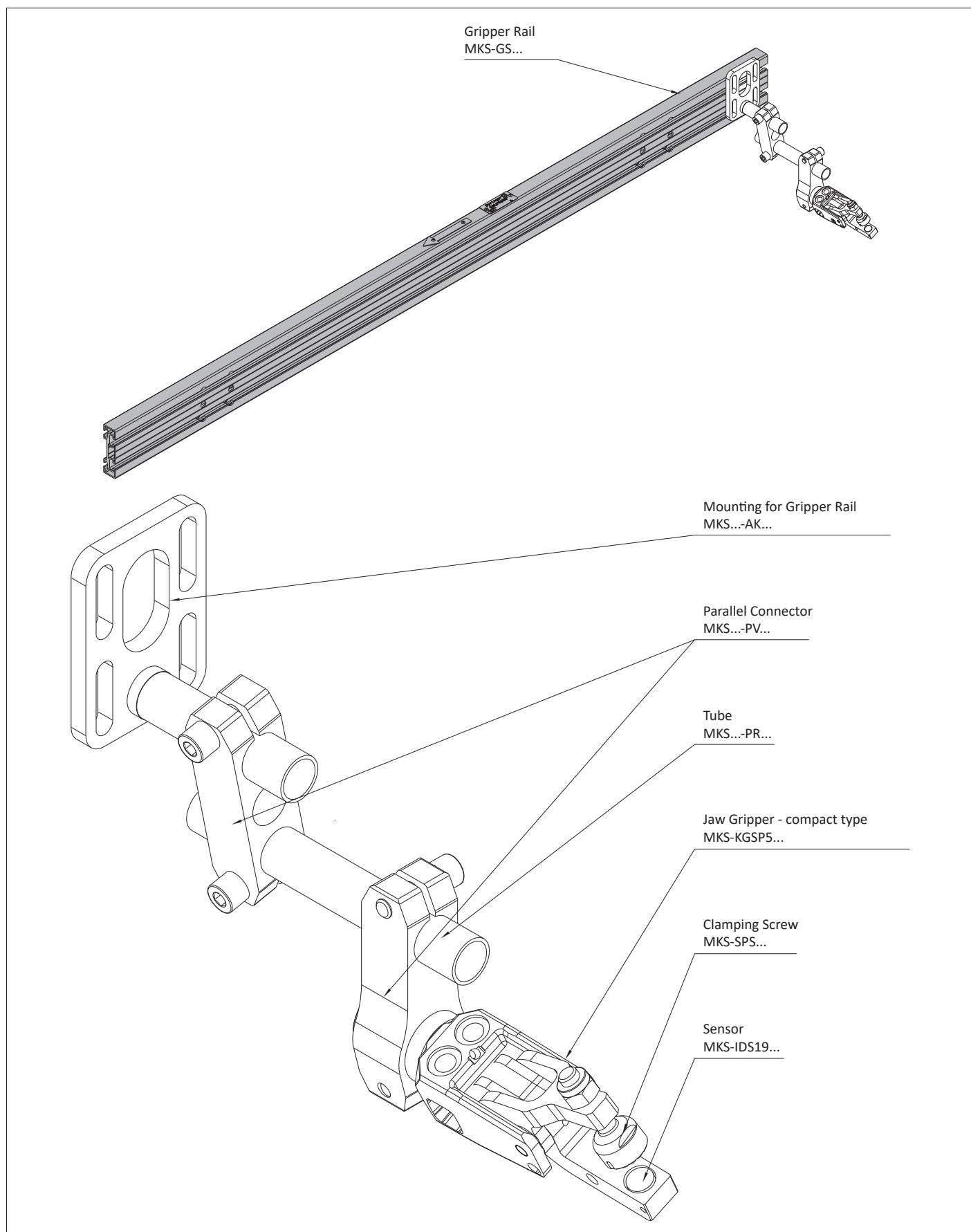
TMZ-Assembly for Tubular with Jaw Gripper
