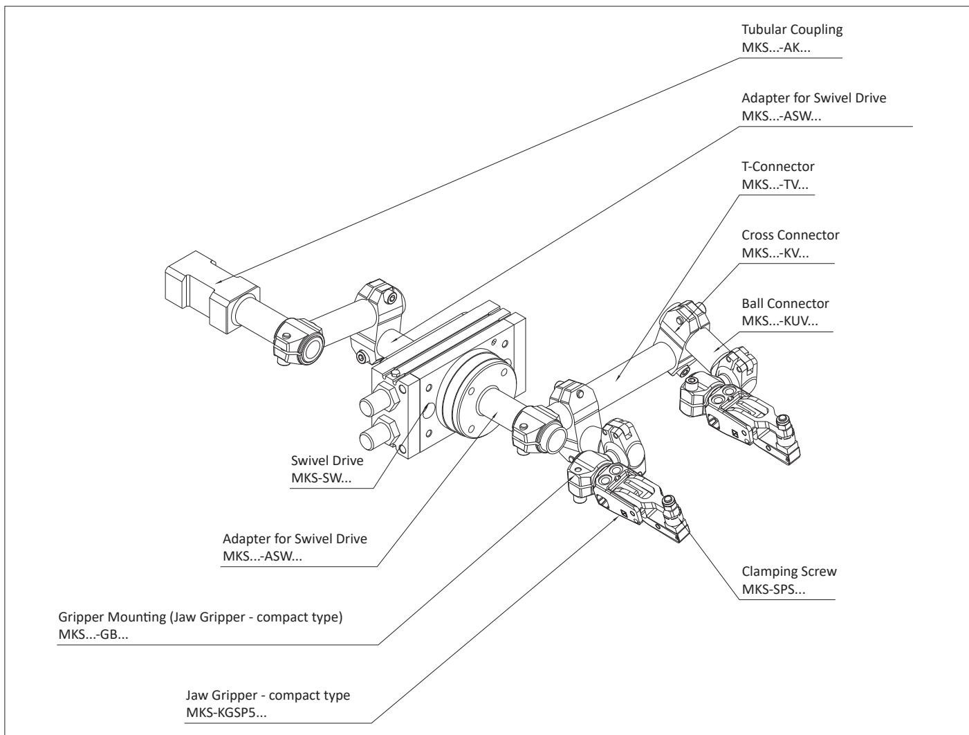
**TMZ-Assembly with Dovetail Coupling and Jaw Gripper (compact type)**
