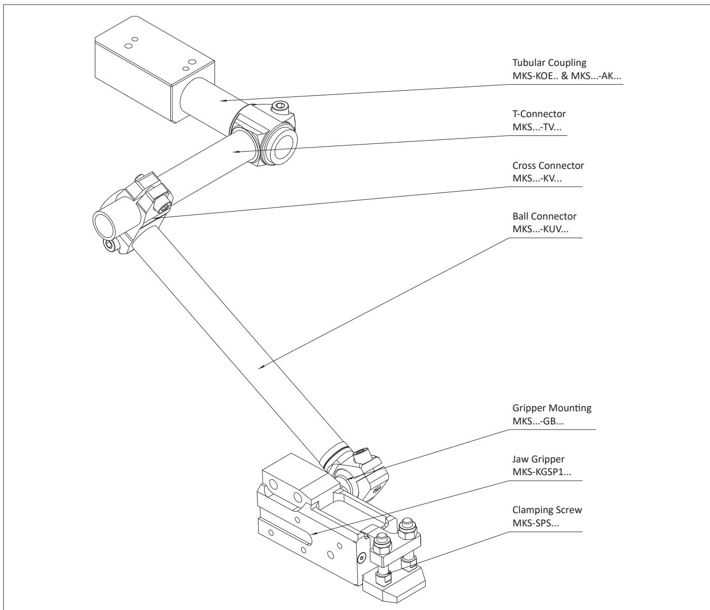
**TMZ-Assembly for Tubular with Jaw Gripper (compact type)**
