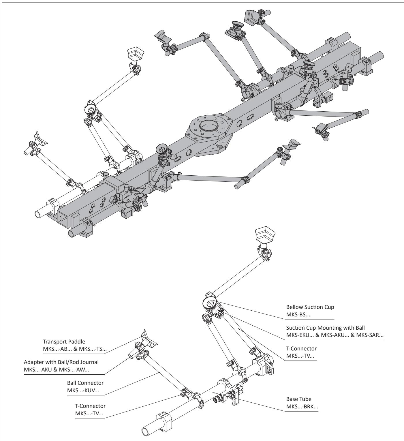
TMZ-Assembly - Tooling with Query (end of line)
