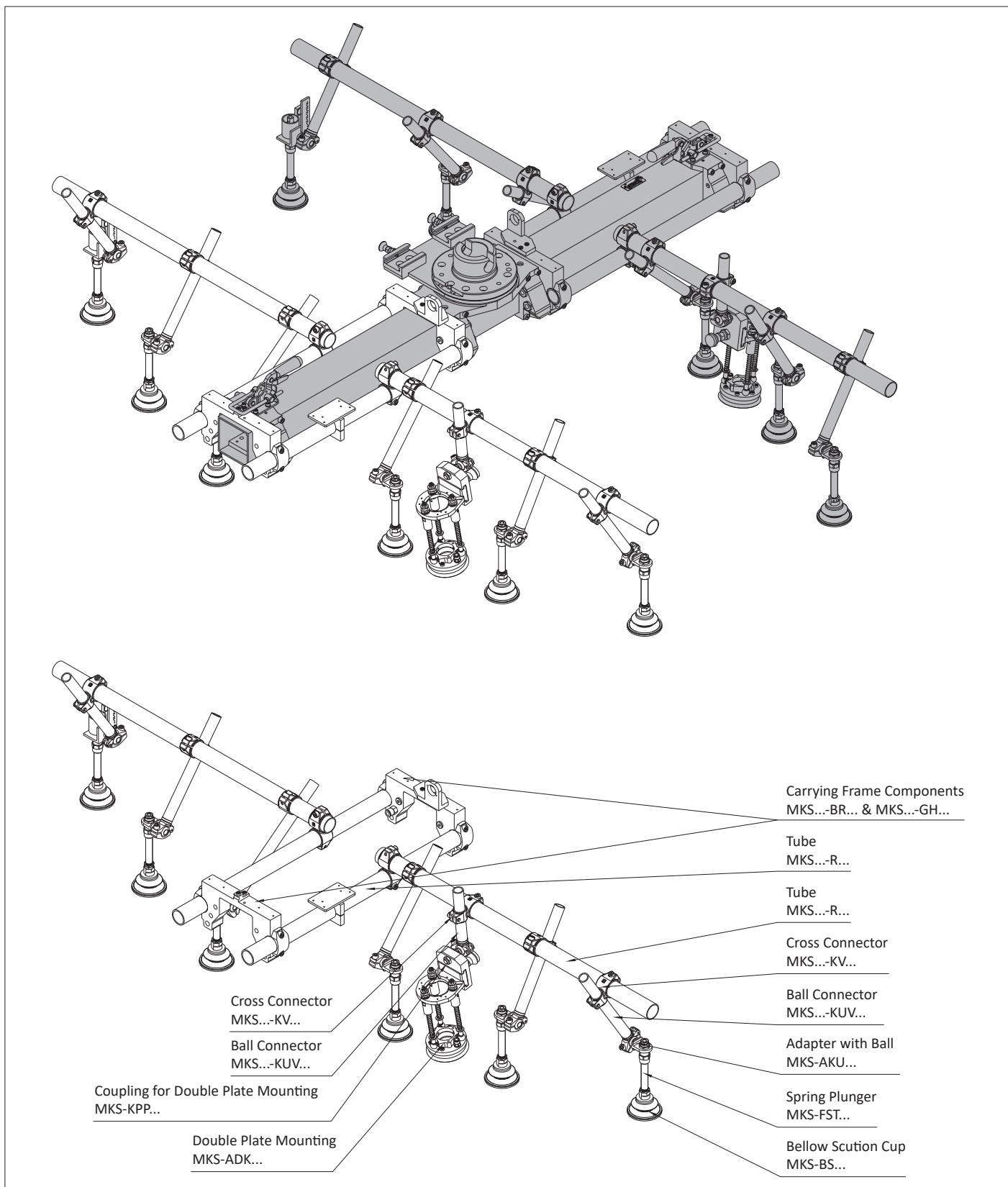
**TMZ-Assembly - Destack-Tooling for Hot Forming**
