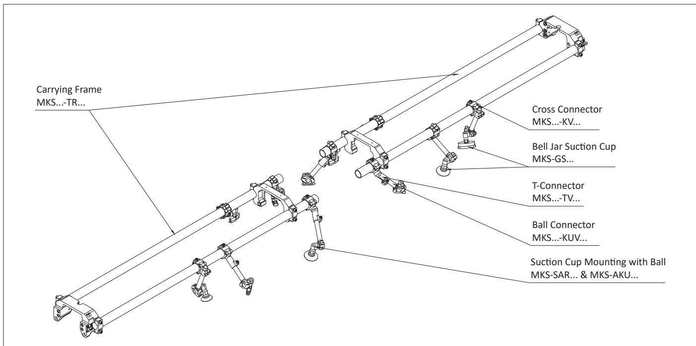
TMZ-Assembly - Unload Feeder for Hot Forming
