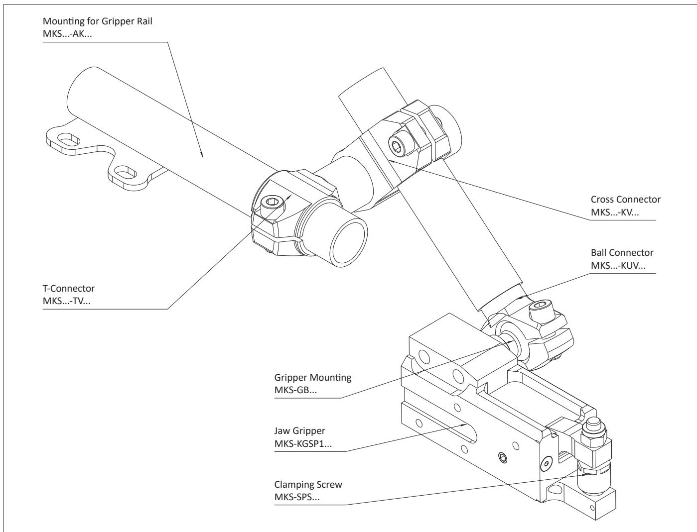
**TMZ-Assembly for Gripper Rail with Jaw Gripper - (compact type)**
