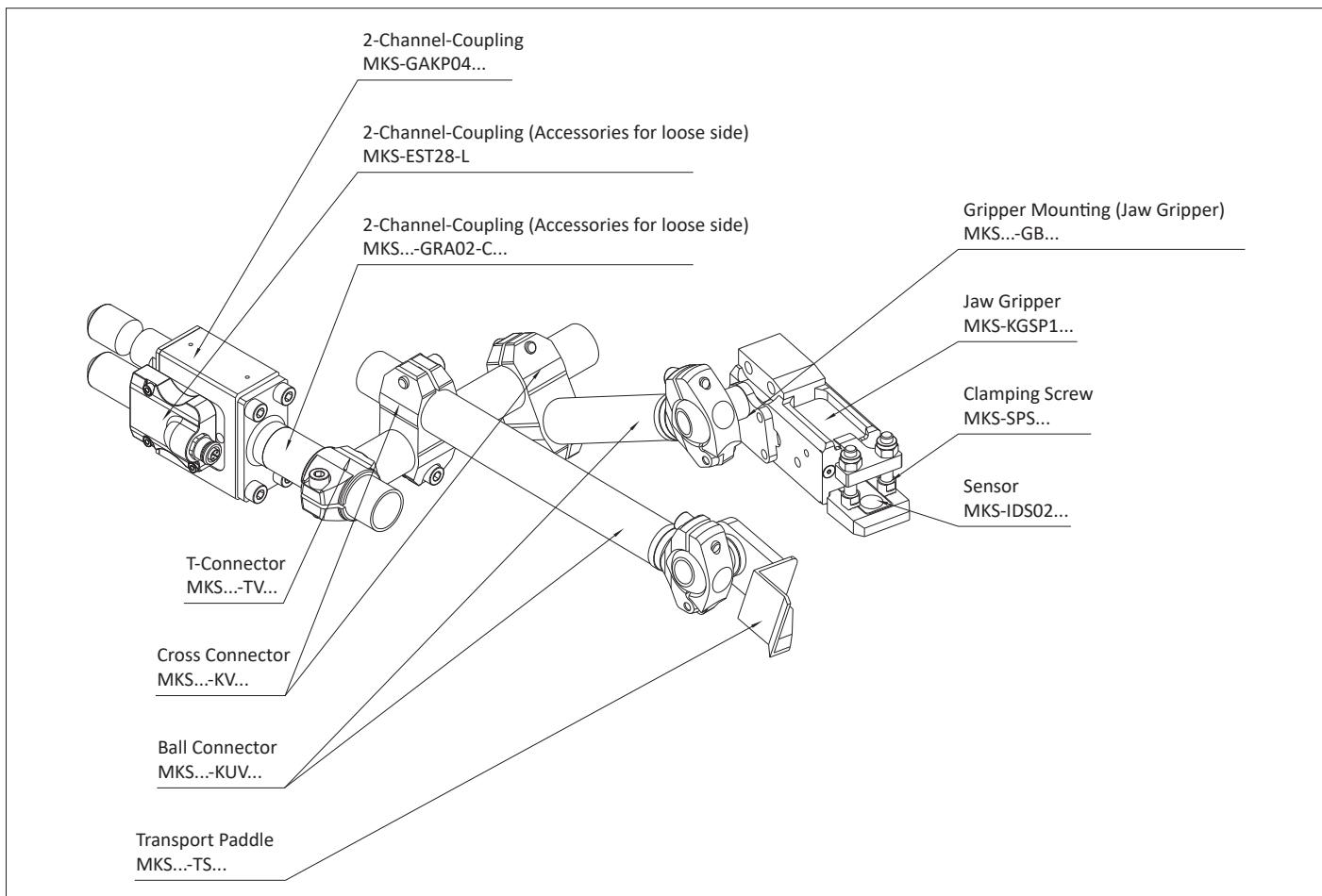
TMZ-Assembly - Double Tube Tooling
