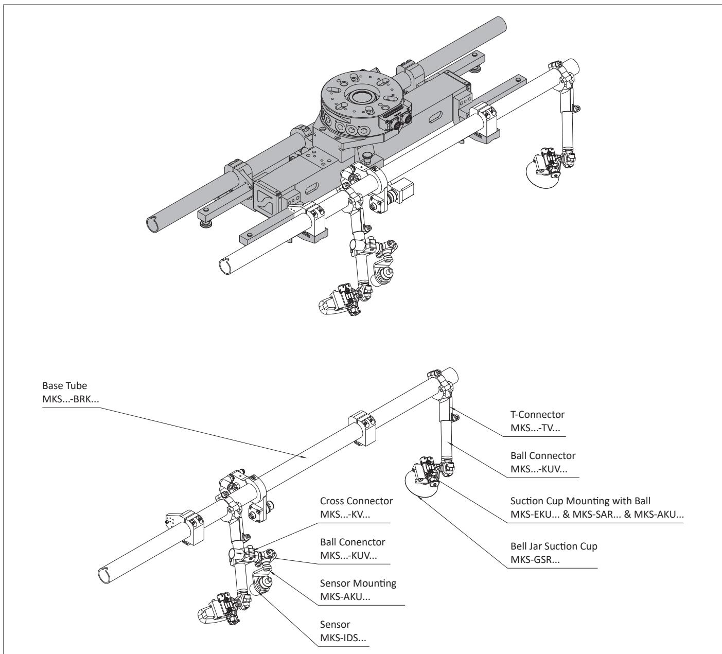
**TMZ-Assembly - Tooling Finished Part Stacking System**
