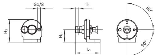
Technical drawings of MKS-SARXX-X showing front view, side view, and top view with 90° rotation capability.
