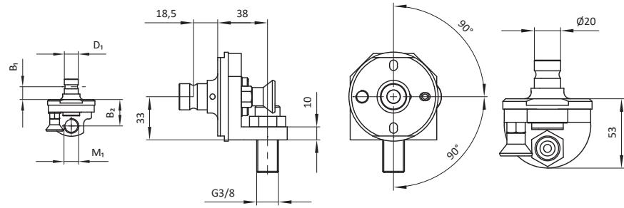
Technical drawings of MKS-SAR28-2 showing front view, side view, and top view with 90° rotation capability.
