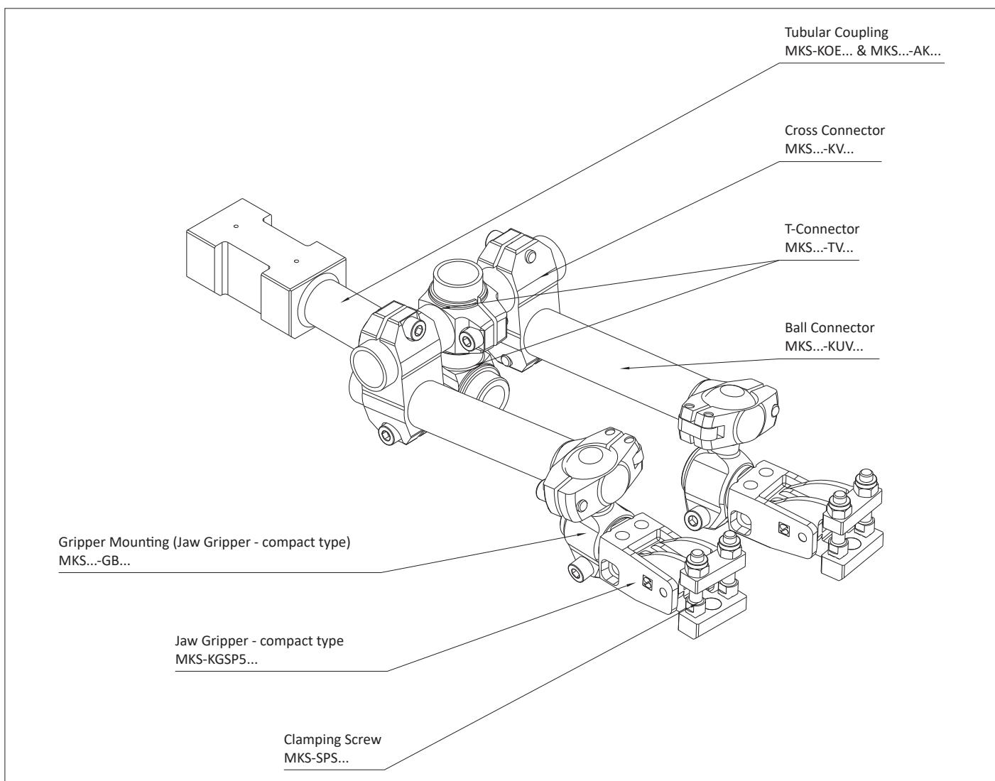
**TMZ-Assembly with Swivel Drive and two Jaw Grippers (compact type)**
